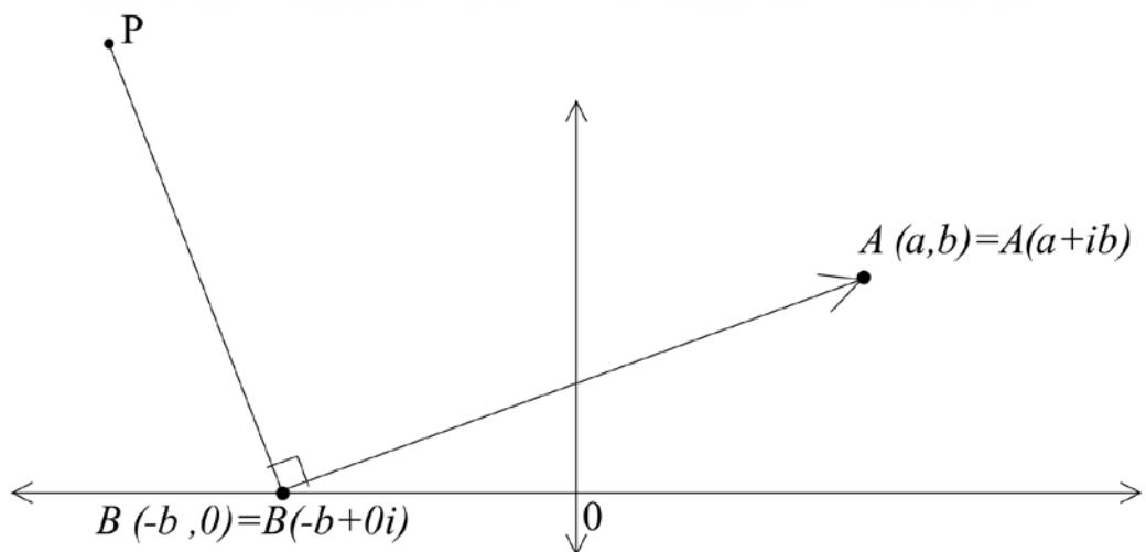
The Argand diagram above shows the point  $A(a,b)$  representing the complex number  $z = a + ib$ , where  $a$  and  $b$  are real.  $B$  is the point  $(-b,0)$ .
