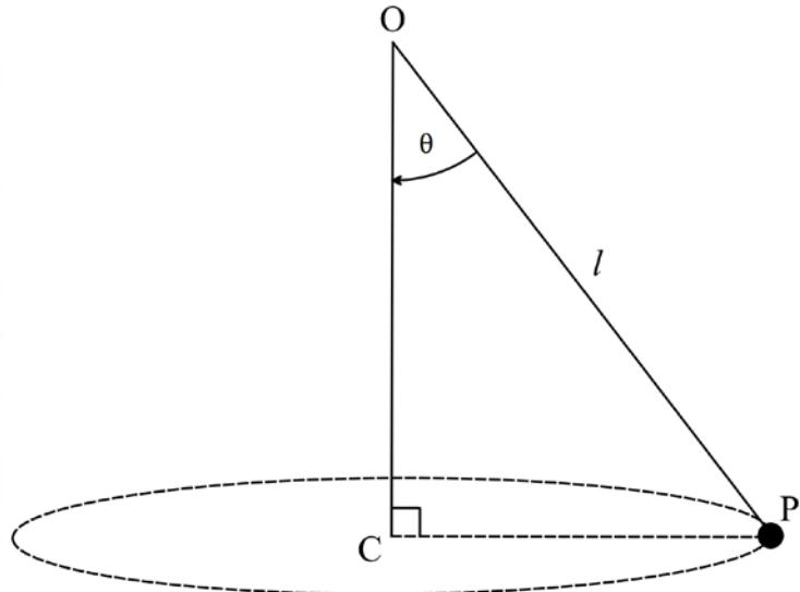
The diagram shows a particle  $P$  of mass  $m$  kilograms suspended from a fixed point  $O$  by a light inextensible string of length  $l$  metres.
